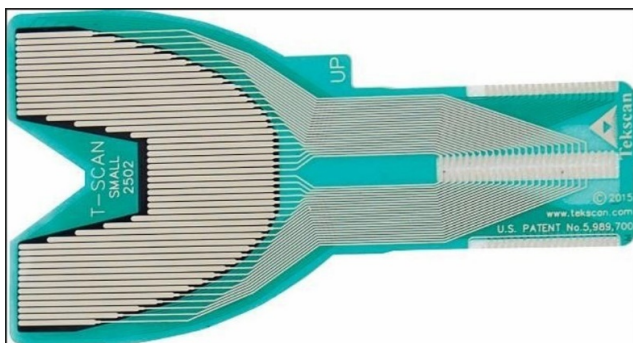
Figure 2D. Small T-Scan HD Novus recording sensor that contains pressure-sensitive conductive ink aligned in columns and rows. The recording matrix transmits occlusal contact force data to the recording handle via the conductive ink rows that run through, and intersect at the end of the sensor tab.
