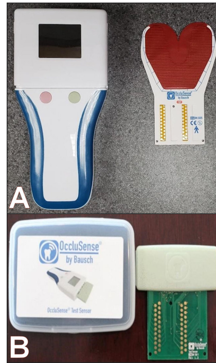
Figure 1A-B. A) Occlusense must undergo a daily Function Test, to establish the handle is working properly. B) The Occlusense recording handle and an unused recording sensor.
