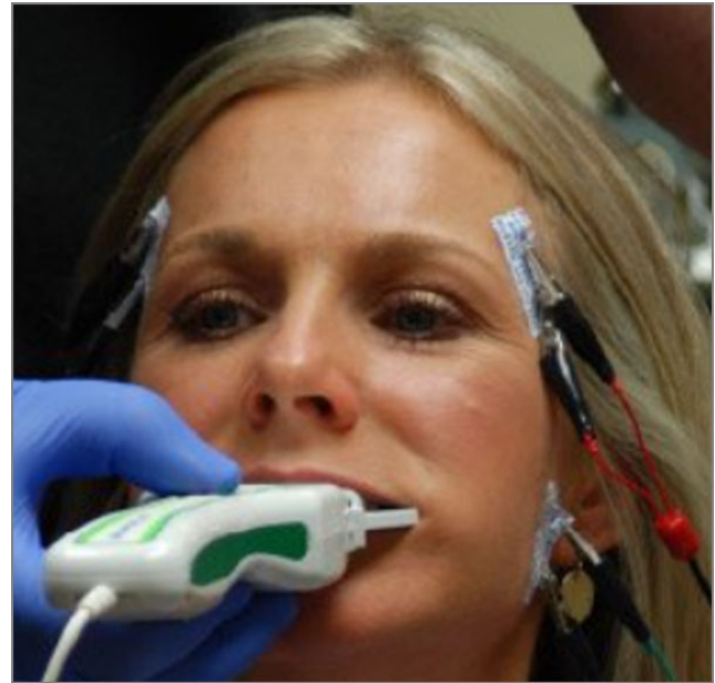
Figure 1. The T-Scan/BioEMG setup that each subject was recorded with. Leads were placed bilaterally on the masseter and temporalis muscles to record muscle activity levels simultaneously with T-Scan force and timing data gathered by the Novus HD recording handle and sensor.
